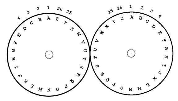
The alphabet runs clockwise round the right wheel and anticlockwise round the left wheel, with the letter 'A' at position number 1 of each wheel. This arrangement can also be represented as below, the letter at the number 1 position always being shown first:
